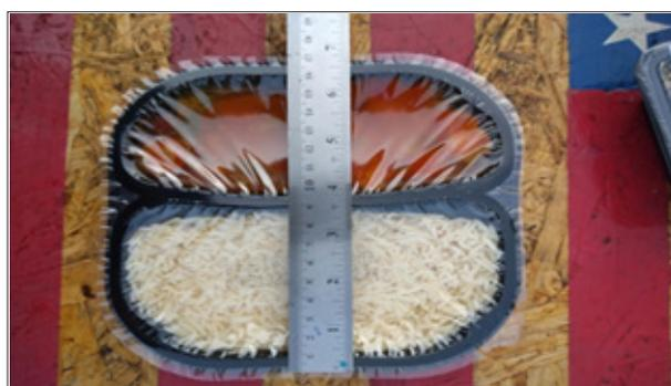
**Figure 2:** Polymeric packaging type C-PET two-section
