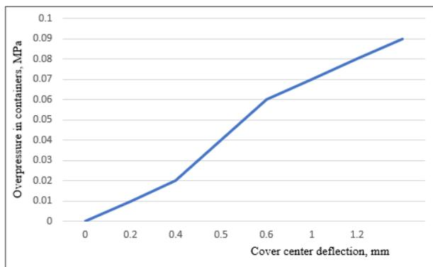
**Figure 4:** Dependence of the deflection of the center of the lid (film) on the magnitude of excess pressure for a metal container with a lid made of polymeric material and a two-section C-PET container
