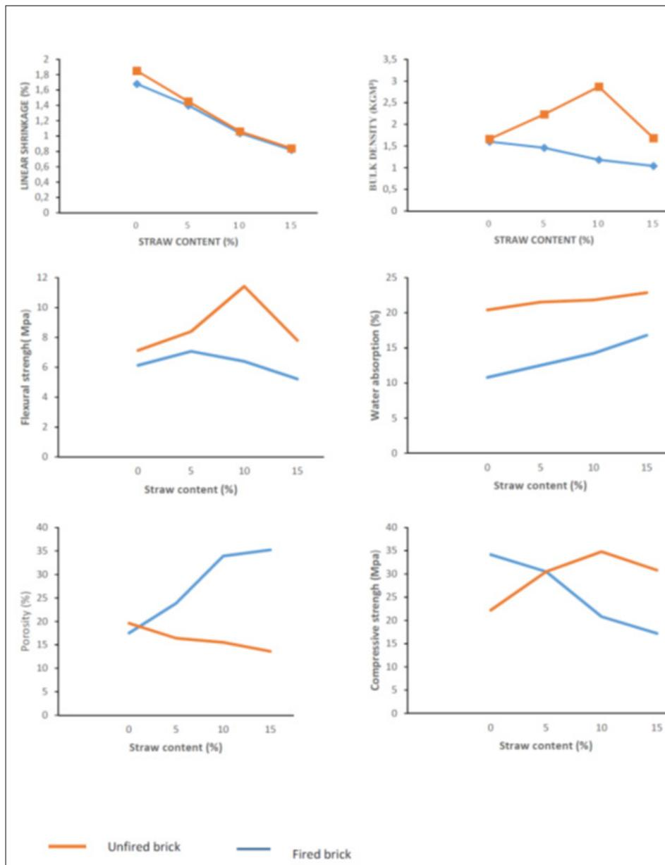
**Figure 6 :** Technological properties of fired and unfired bricks with straw addition
