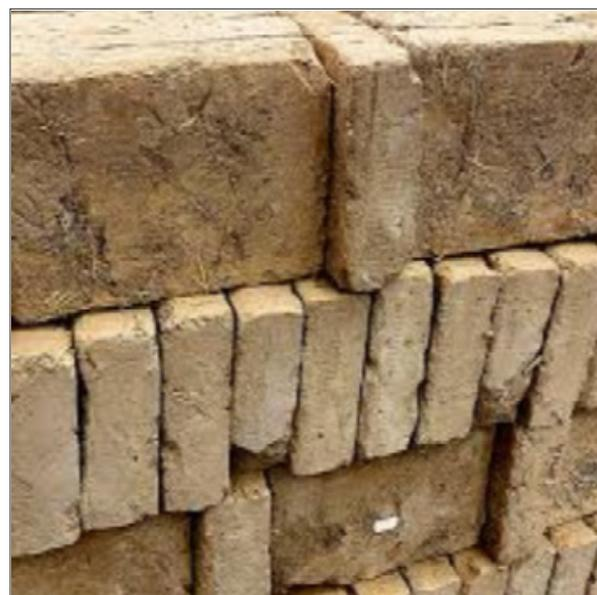
**Figure 5 :** Unfired brick with straw addition
