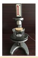
**Figure 1:** Experimental set up. Kidney specimen is placed on Petri dish. LEDs (shown with arrow) are placed under the specimen. CCD camera (shown also with arrow) is connected to PC. IR passing through tissue carries information about optical density inhomogeneity caused by existence of cancerous formations.
