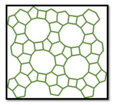
Figure 2: Simulated and simplified structure of zeolite EMM-17
