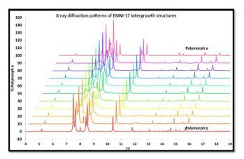
**Figure 9 :** DIFFaX simulated diffraction patterns for intergrowths of EMM-17 polymorphs A and B at successive 10% intergrowth intervals. The bottom scan is 100% polymorph B and the top scan is 100% polymorph A [22]
