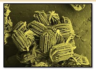
Figure 6 : SEM picture of EMM-17 prepared with OSDA3 showing rolodex morphology.[22]
