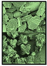
Figure 7: EMM-17, a New Three-Dimensional Zeolite with Unique 11-Ring Channels and Superior Catalytic Isomerization Performance [22]
