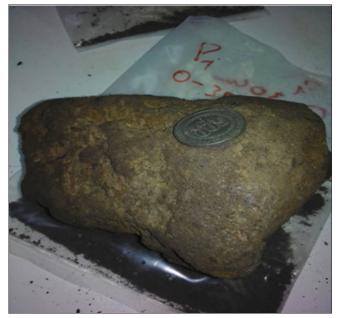
Figure 3: Meskine Clay sample
