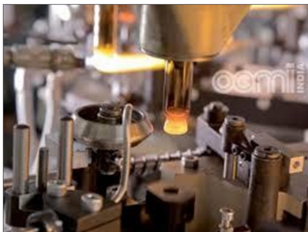
Neck & bottom formation of Tubular Glass vial (beginning)
