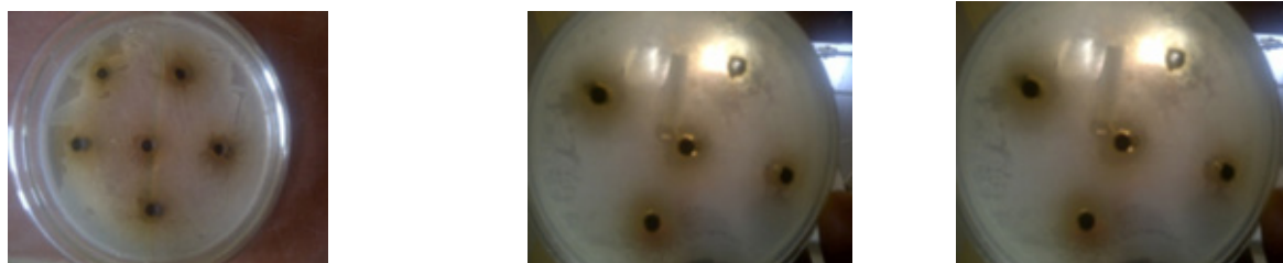
d) O. gratissimum against E. coli ATCC 11775 e) O. gratissimum against S. aureus ATCC 6538 f) O. gratissimum against C. albicans ATCC 10231
