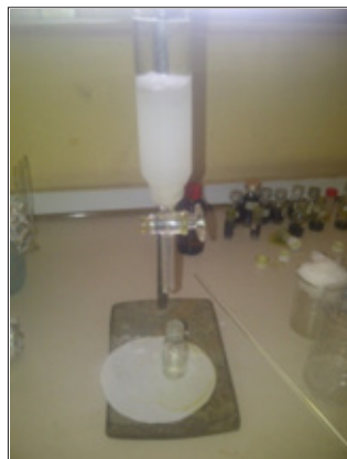
(i) Column packed with silica gel
