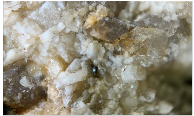
Figure 5 : The texture of the granite of an ashlar from the Monastery of El Escorial (Spain), seen with a 50X magnifying glass (photo by the author).
