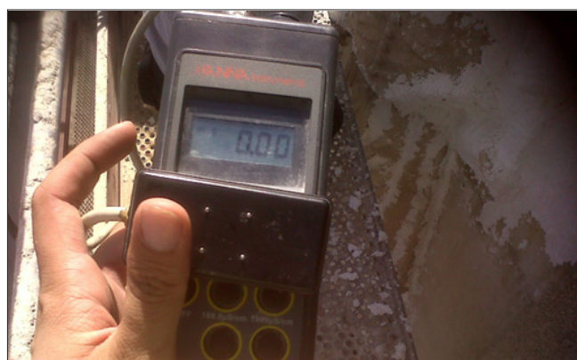
Figure 12: Equipment used for the measurement of conductivity and, therefore, for the measurement of salts in the Patio de Santo Tomás of the University of Alcalá de Henares, in Spain (photo by author).
