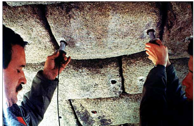
Figure 15: Auscultation of the ultrasonic transmission speed in the ashlars of the Roman Aqueeduct of Segovia (Jurado, 2002)
