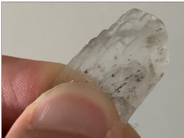
Figure 6: Crystallized gypsum, which can be scratched with a fingernail (photo by the author).
