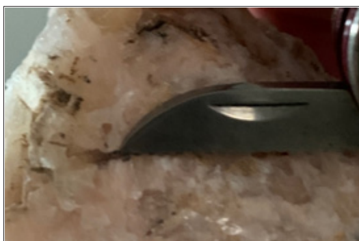
Figure 7: Limestone and dolomite are sedimentary rocks that can be scratched with a knife: to differentiate the two, we often need to resort to the use of acids (photo by the author).
