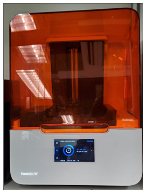
Figure 6: Operation of the SLA 3D printer Form3B+. The final model was designed and sent to the 3D printer to proceed on fabrications.
