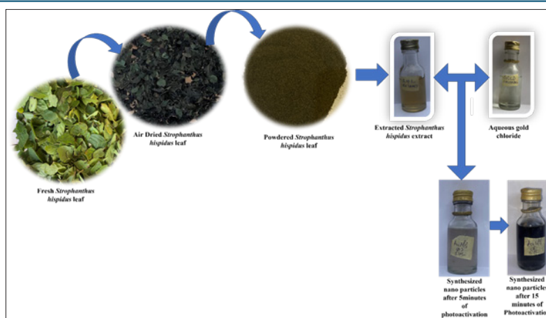
Figure 1: Sample preparation and green synthesis of gold nanoparticles from Strophanthus hispidus leaf
