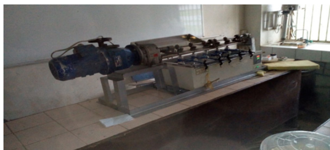
Figure 1: The fermentor used for liquefaction and saccharification
