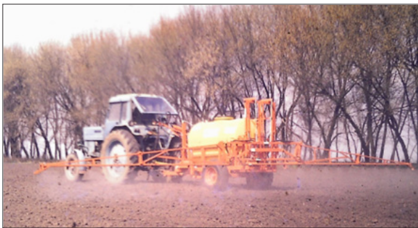
Figure 6: Tractor with trailer spray tank and boom.
