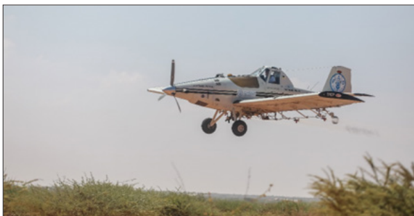
Figure 11: Using aircraft to spray biopesticide.
