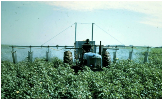
Figure 5: Tractor mounted sprayer applying insecticide on cotton crop.
