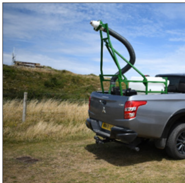
Figure 10: Rotary atomiser on truck mounted sprayer.
