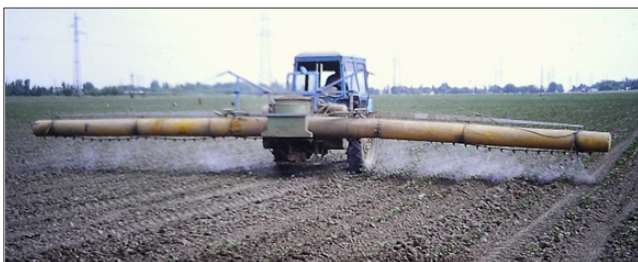
Figure 7: Tractor with air assisted distribution of spray.
