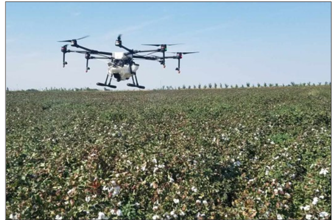
Figure 8: Drone spraying cotton in China.
