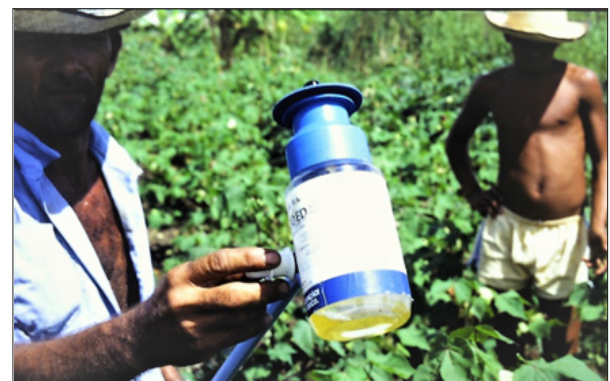
Figure 16: A hand-held electrostatic sprayer that was used in Brazil on cotton. It was withdrawn as it needed less active ingredient to provide effective control.
