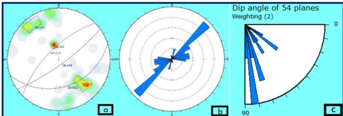
Figure 5: Stereonets of cyclograms (a) and directional poles and rose diagram (b) and dips (c) of all stratification planes.
