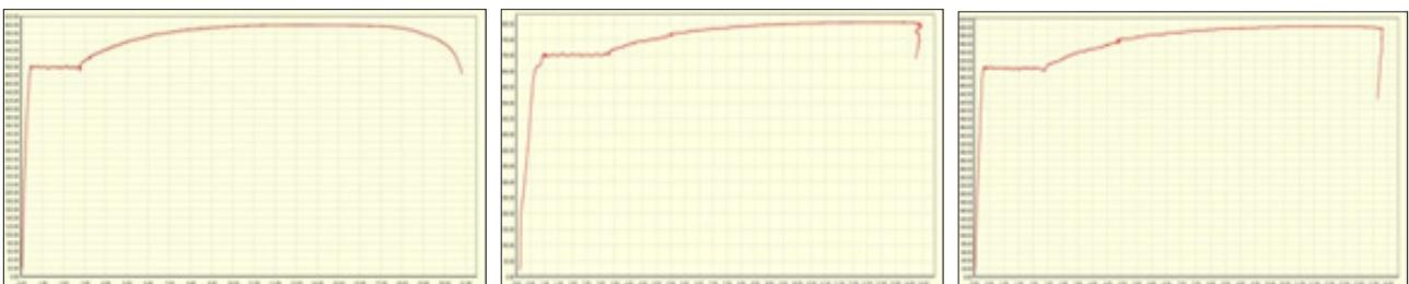
**Figure 6:** Stress (y-axis)-strain (x-axis) curves shape of the steel rebars intermittently sprayed with a constant amount of 3.5% NaCl solution and after two minutes placed in an oven at 100°C.
