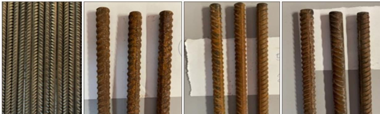
**Figure 1:** Steel rebars exposed to a 3.5% wt. NaCl solution and after the exposition to an increasing temperature (from left to right).
