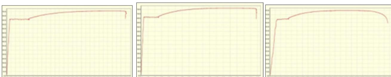
**Figure 3:** Stress (y-axis)-strain (x-axis) curves shape of the reference steel rebars.
