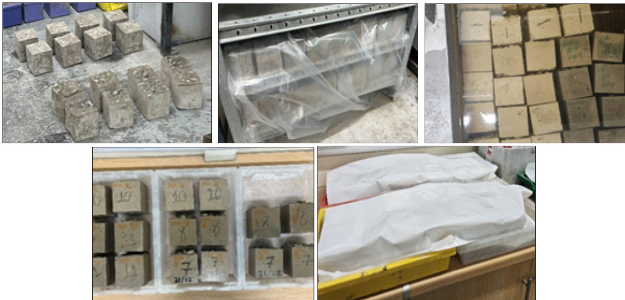
Figure 3: (a) 100 x 100 x 100 mm Specimens (b) Prevention of Alkaline Solution Evaporation (c) Water Curing (d) Air Drying (e) Air Curing
