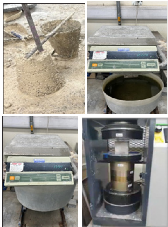
Figure 4: Geopolymer Concrete Specimens (a) Under Slump Testing (b) Under Density Testing (Mass Dry) (c) Under Density Testing (Mass Wet) (d) Under Testing of Compressive Strength
