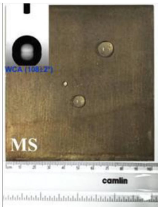
Figure 13: Photographs of hydrophobic GZH-10 coated MS sheet (size: 100 mm x 100 mm).
